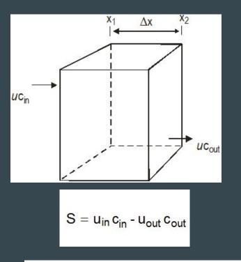
In an empty chamber (no sources or sinks)  $F_{in} = F_{out}$  and  $\Delta c/\Delta t = 0$ .
