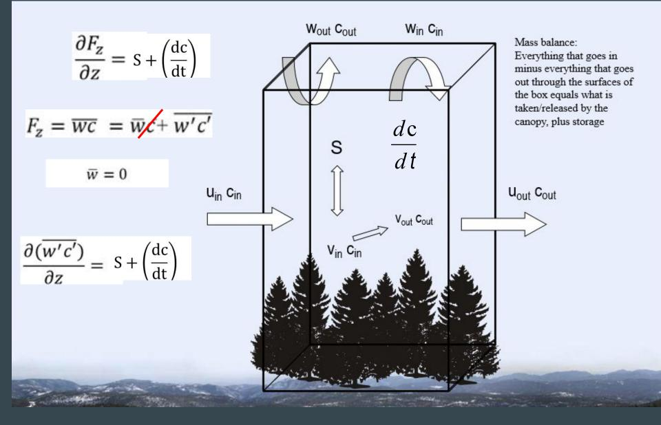
$$\frac{\partial(\overline{w'c'})}{\partial z} = S + \left(\frac{dc}{dt}\right)$$
