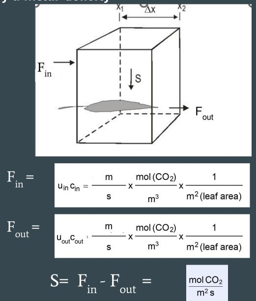
Alternatively, the flux can be expressed as an air speed (flow speed multiplied by a molar density:
