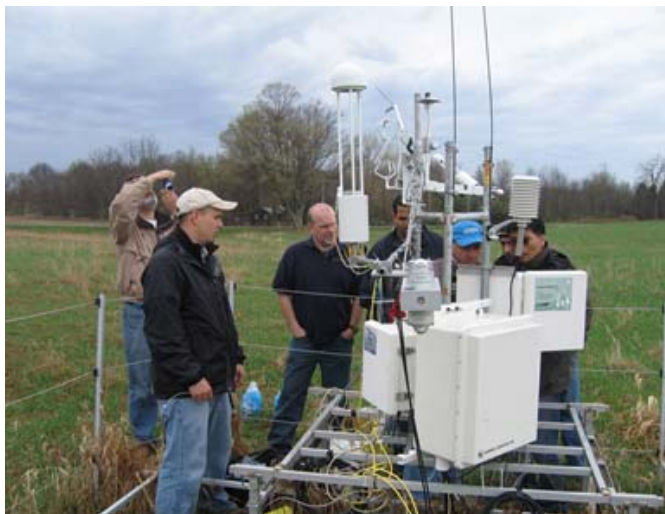
Photo 1: The J-Rover developed for the bioenergy study at the GLBTRC/KBS site in Michigan was enhanced to include a CH 4 sensor (LICOR 7700) in May 2010.
