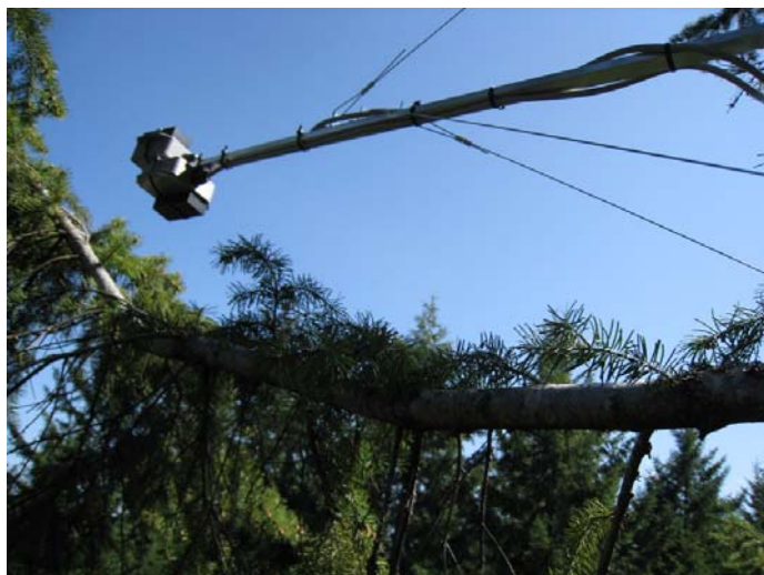
Figure 2 - PRI Sensors mounted in a Douglas-fir forest canopy, Campbell River, British Columbia, Canada. Sensors based on a design by Garrity et al. 2010. Photo courtesy Martin van Leeuwen.
