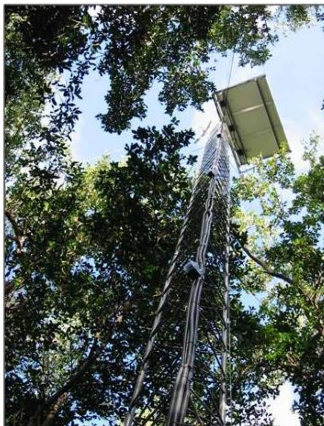
Figure 2: The eddy covariance tower, seen here before Hurricane Wilma, extends ~10 m above the 20 m tree tops and is supported by a wooden platform built on a peat substrate 5 to 6 m thick.
