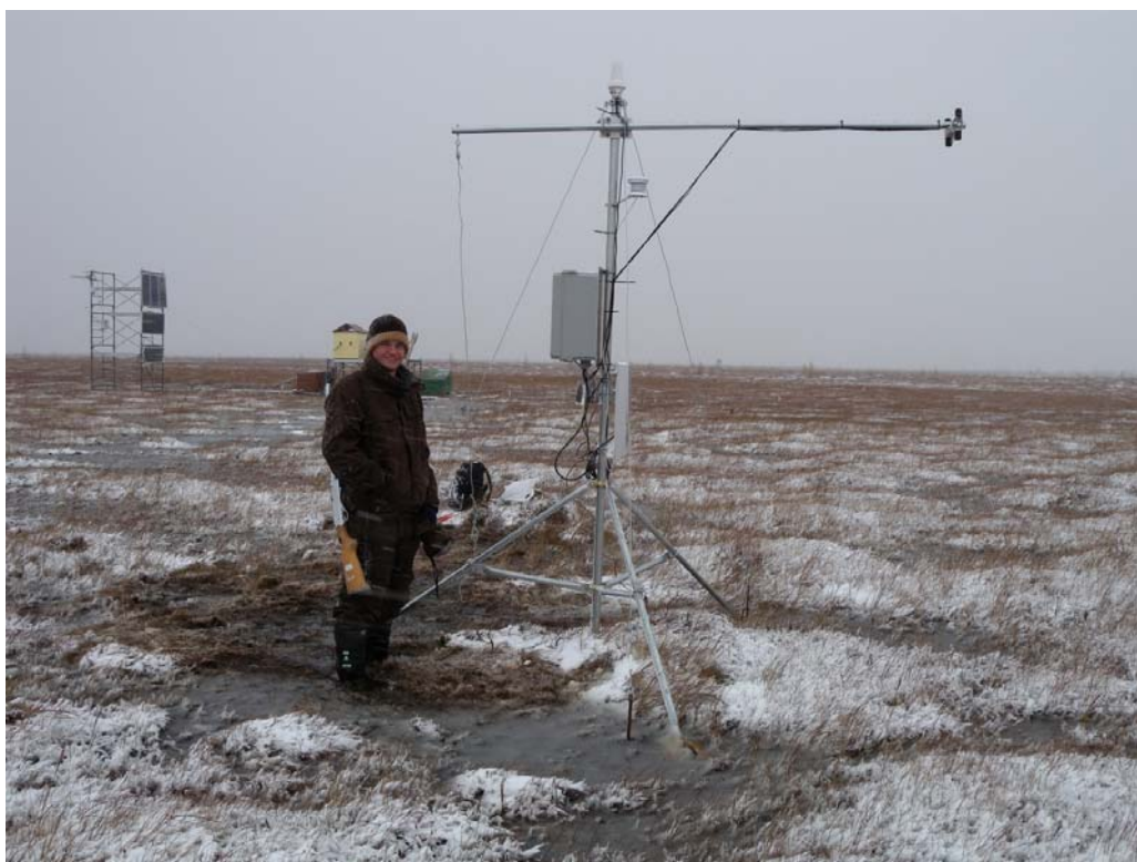
Figure 1 - “Phenology station” sampling NDVI in a fen site, Churchill, Manitoba, Canada. Note the flux tower in the background (operated by M. Tenuta, University of Manitoba).
