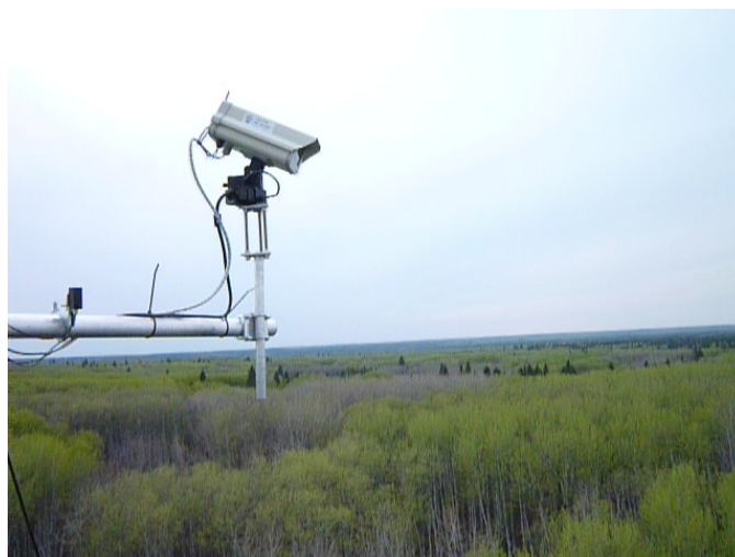
Figure 5 - AMSPEC II system combining a webcam with multi-angle spectral reflectance measurements of the Southern Old Aspen site, Saskatchewan, Canada. Photo: Thomas Hilker.
