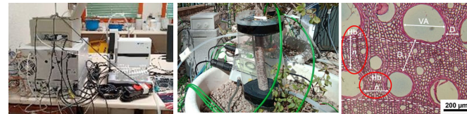
From the upper left to the lower right photo: Delta Ray IRIS to measure 18 O and 13 C isotopes of gaseous CO 2 ; stem CO 2 chamber; xylem anatomical variables.
