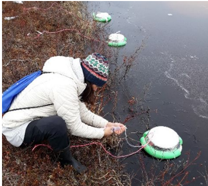
Theresia Yazbeck takes chamber measurements near site CA-TVC in the Arctic tundra while working with Oliver Sonntag at the Université de Montréal, Canada. There she worked on modeling the site's carbon flux with the ELM land surface model.
