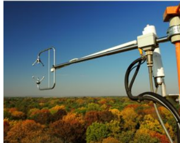
Eddy Covariance (EC) system installed on top of the tower in ICOS class 1 station (CZ-Lnz)
