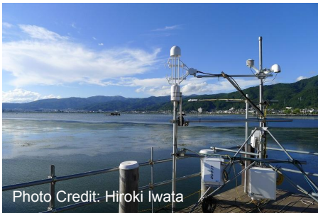
Photo Credit: Hiroki Iwata The observation mast installed at Lake Suwa. Campbell CSAT3 sonic anemometer and Li-Cor LI-7700 \text{CH}_4 analyzer are used for the flux observation.
