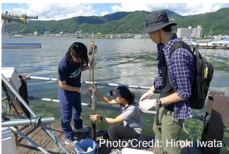
Photo Credit: Hiroki Iwata Students sampling a sediment core. The sediment core was used in an incubation experiment for \text{CH}_4 production.
